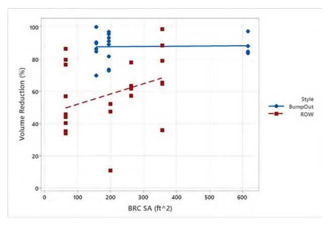
Figure 16: Volume reduction as a function of bioretention cell (BRC) surface area for practices constructed in the right-of-way (ROW) or as bump-outs (BMPOUT) into roadside parking areas.
