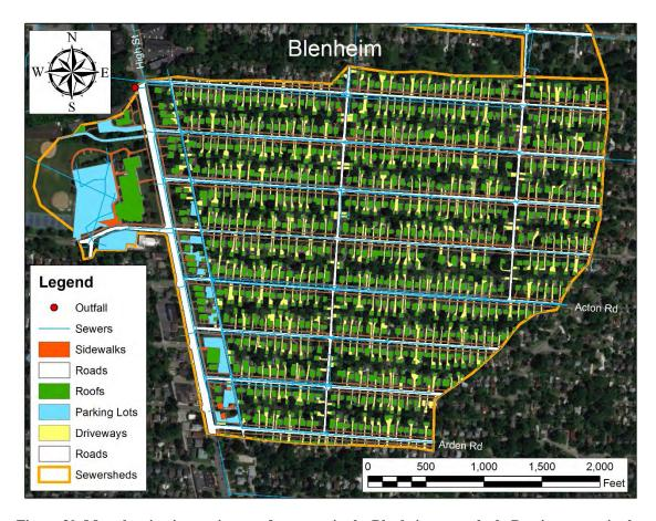
Figure 30. Map showing impervious surface types in the Blenheim sewershed. Pervious areas in the sewershed are not highlighted with color.
