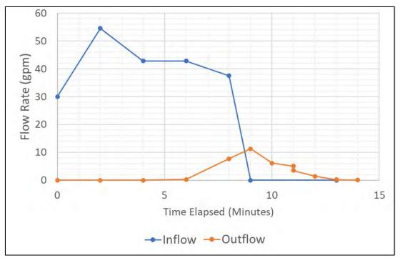
Figure 14. Inflow and outflow hydrographs from simulated storm testing performed at a bioretention cell in the Indian Springs sewershed (270 Village Dr). The increase in inflow rate between 0 and 2 minutes reflects the full opening of the valve after the test began, which more commonly occurred immediately after tests commenced.
