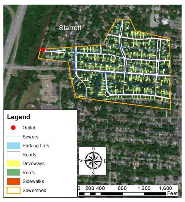
Figure 31. Map showing impervious surface types in the Starrett sewershed. Pervious areas in the sewershed are not highlighted with color.
