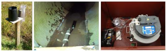
Figure 5. Rain gage cluster (left), sample intake (clear plastic) and area velocity meter (black) in the Cooke-Glenmont outfall (center), and automated sampler at Beechwold (right).
