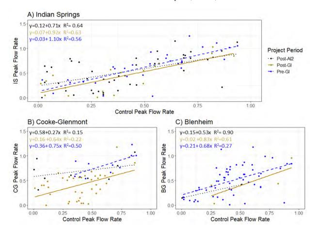
Figure 13. Area normalized peak flow, also referred to as areal peak discharge (in/hr), in the treatment sewersheds compared to the control (Beechwold). Note that data from the monitored sewersheds have been log transformed. Changes in slope indicate differences in the normalized peak flow relationship between the control and treatment sewershed between the pre-GI and post-GI (or post-AI²) project phases.
