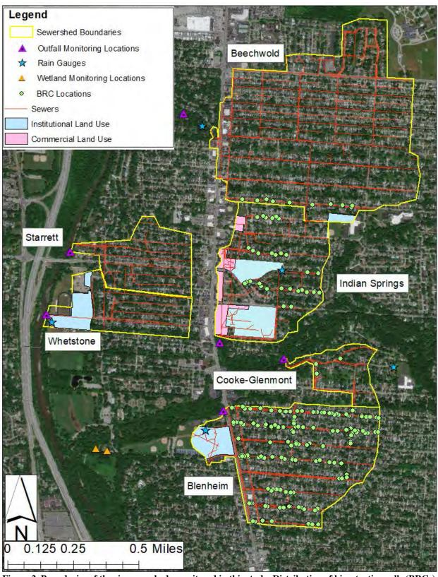
Figure 2. Boundaries of the six sewersheds monitored in this study. Distribution of bioretention cells (BRCs), monitoring locations, and land use within each sewershed also shown. The remaining area within each sewershed not identified as commercial or institutional is residential.
