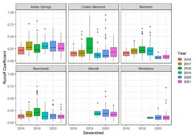
Figure 9: Yearly changes in the distribution of runoff coefficients in the six monitored sewersheds between 2016-2021.
