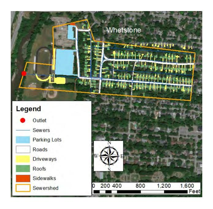
Figure 32. Map showing impervious surface types in the Whetstone sewershed. Pervious areas in the sewershed are not highlighted with color.
