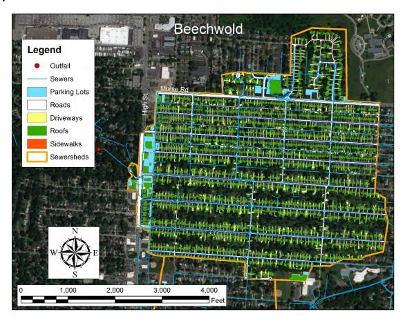
Figure 27. Map showing impervious surface types in the Beechwold sewershed. Pervious areas in the sewershed are not highlighted with color.
