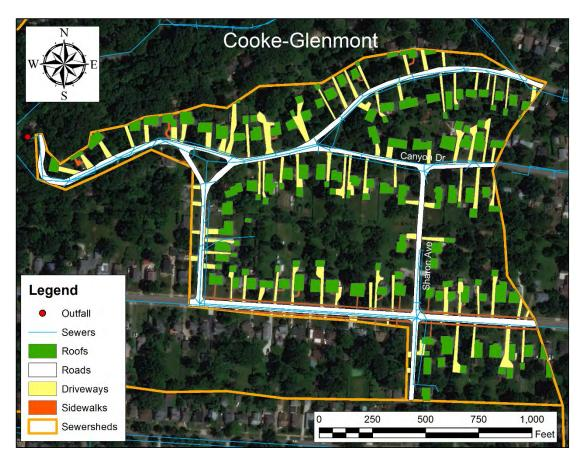
Figure 29. Map showing impervious surface types in the Cooke-Glenmont sewershed. Pervious areas in the sewershed are not highlighted with color.
