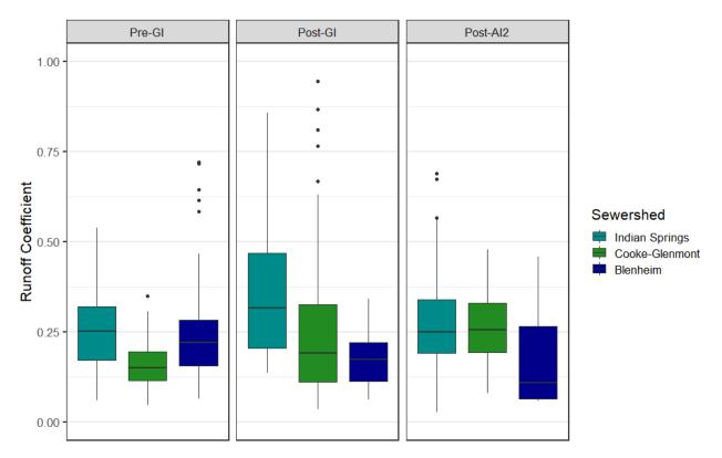
Figure 12: Distribution of runoff coefficients during storm events in each of the treatment sewershed by project phase.
