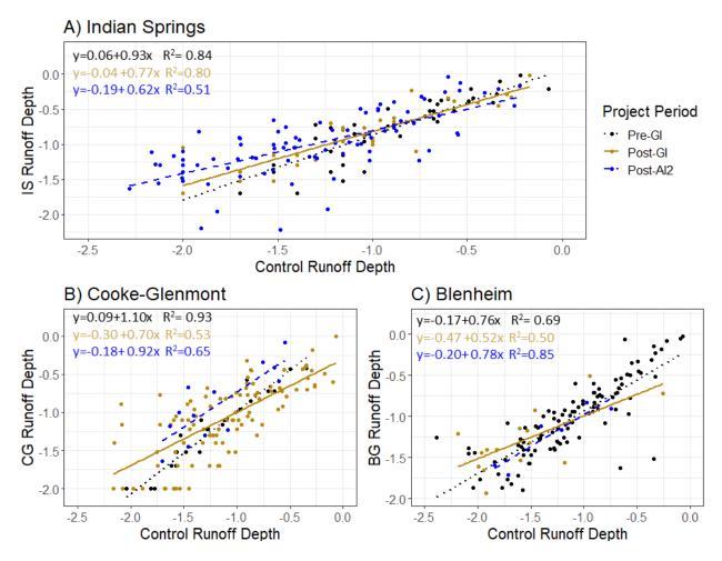
Figure 10. Runoff depth relationships for the treatment sewersheds and control (Beechwold) during the various project periods. Note: runoff depths are log transformed. Changes in slope indicate differences in the runoff depth relationship between the control and treatment sewershed between the pre-GI and post-GI (or post-AI $^2$ ) project phases.
