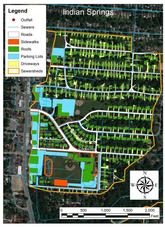
Figure 28. Map showing impervious surface types in the Indian Springs sewershed. Pervious areas in the sewershed are not highlighted with color.
