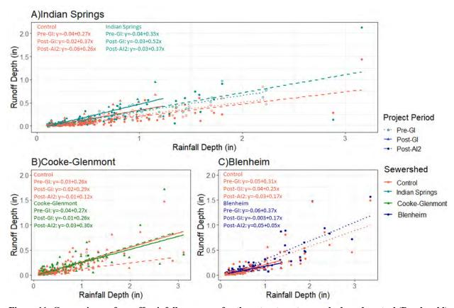
Figure 11: Comparisons of runoff-rainfall responses for three treatment sewersheds and control (Beechwold) for all project phases.
